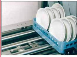
can be disconnected in a matter of seconds moved away to allow full access to the dishwasher. The rollers themselves can easily be removed from the table bed for cleaning. An investment in a COMENDA dishwasher mechanised system ensures prompt payback as well as systemic efficiency.
