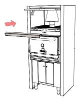
An alternative option to provide more working space inside the heating cabinet is to install the security accessories outside of the cabinet. In order to do this, connect the extended flue duct to the oven smoke outlet prenetrating the cabinet's roof. Assemble the firebreak and dissipating filter over the duct.
